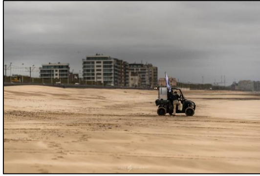
Figure 1-7. Topographical survey with a mobile laser scanner on the beach of Mariakerke-Bad, September 2016.
