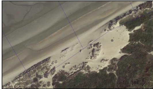
Figure 3-15. Dune blowouts at sections 36 to 38.
