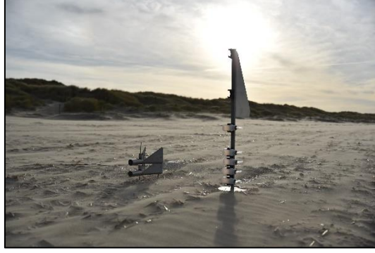
Figure 5-4. The Modified Wilson And Cook sand trap (MWAC) and saltiphones, measuring sand transport on the beach of Koksijde, 24 November 2016. Note the presence of different sized shell fragments.
