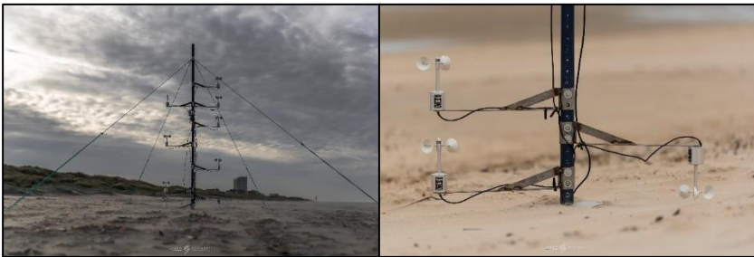
Figure 1-4. Combined meteorological station with eight anemometers, a wind vane and a temperature sensor.
