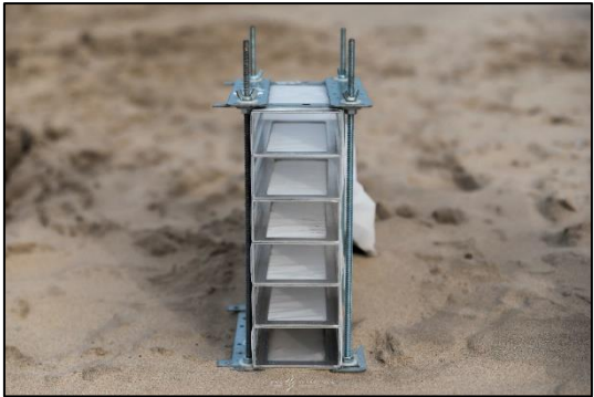
Figure 2-8. Vertical mesh sand trap covering a height of 30 cm. Image taken on 24/11/2016 on the subaerial beach of Koksijde.
