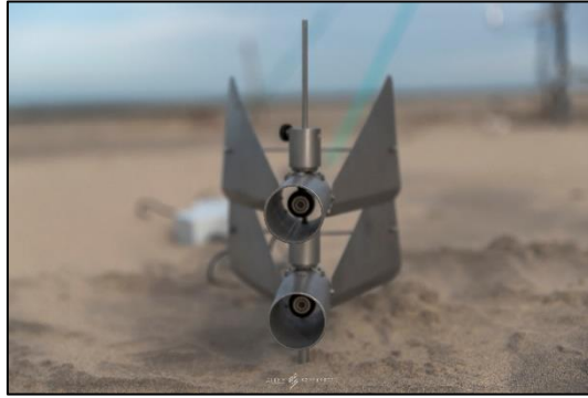
Figure 1-6. Array of saltiphone sensors during an aeolian measurement campaign on the beach of Mariakerke-Bad, November 2016.
