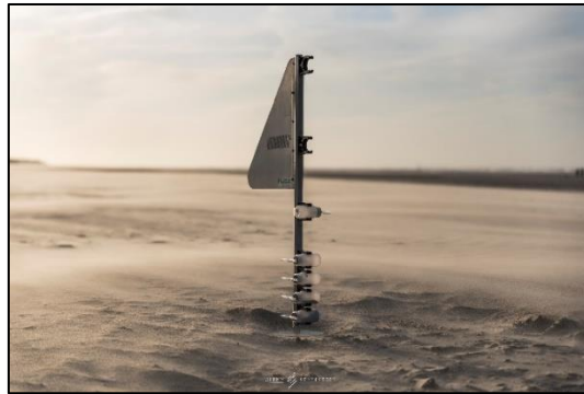
Figure 1-5. The Modified Wilson And Cook sand trap (MWAC), measuring sand transport on the beach of Koksijde, November 2016.
