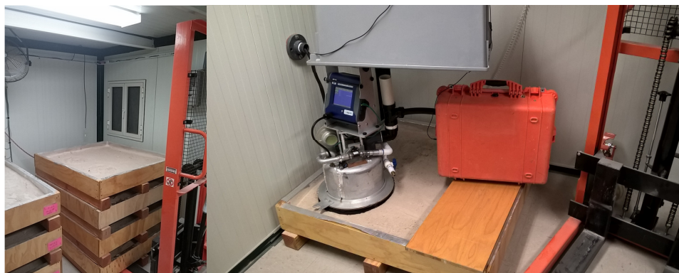
Figure 1. Ash samples in condition chamber (left) and ash sample undergoing PI-SWERL tests (right).
