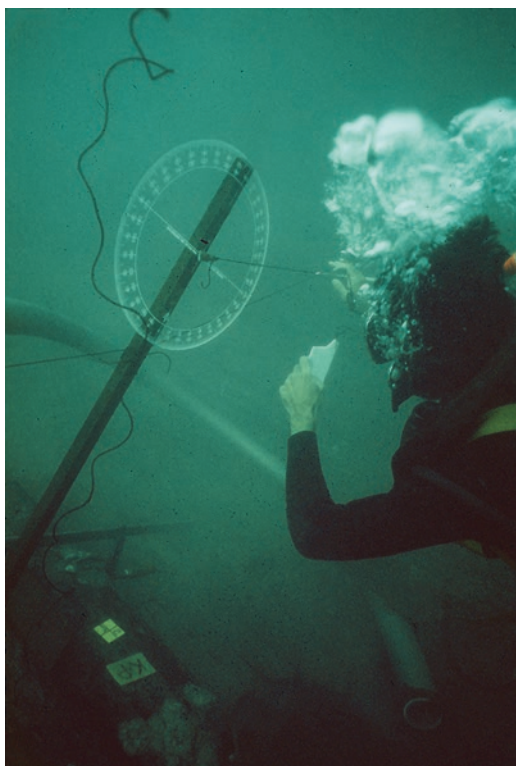
Fig. 3.10 Circular protractor used to record profiles
