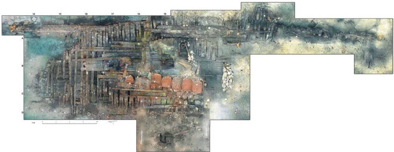
Fig. 4.11 (a and b) Composite photogrammetric 3D model of the research campaigns 2015 and 2016, and the respective orthomosaic (K. Yamafune, R. Torres, S. Govorčin, D. Gorički)
