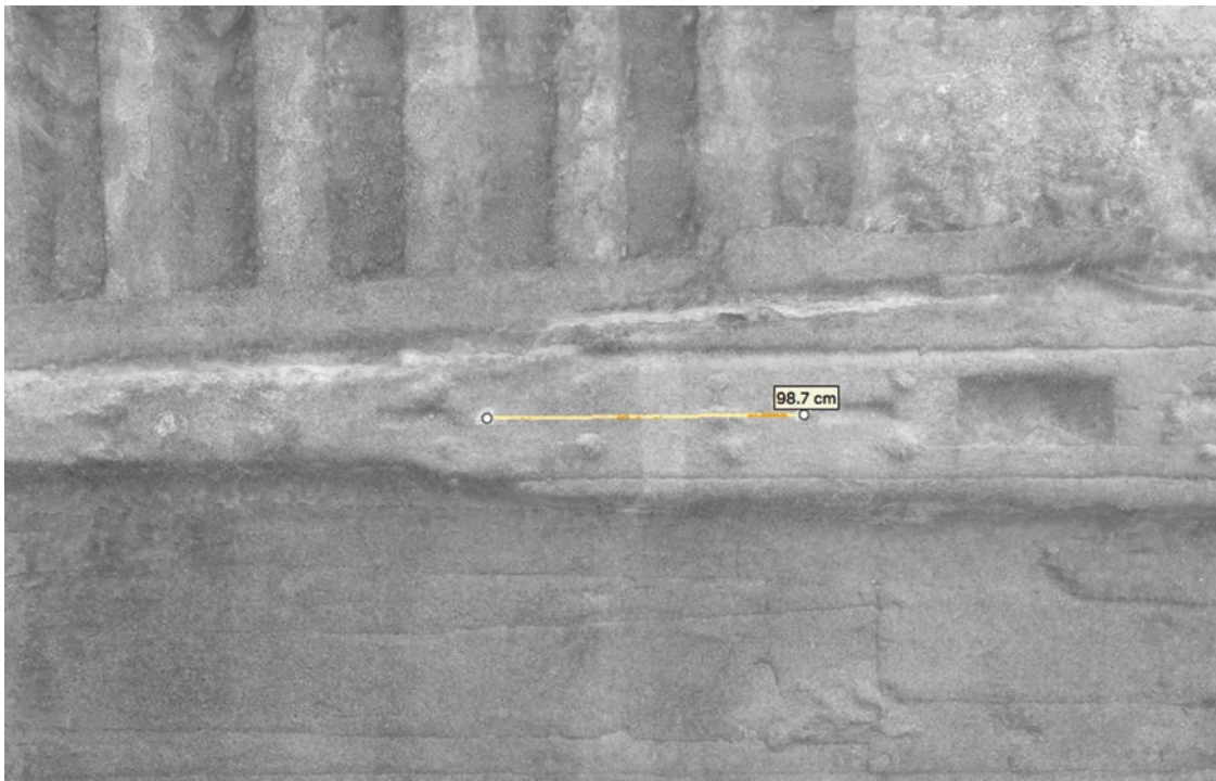
Fig. 3.16 Detail of PhotoScan/Metashape model of Santo António de Tanná keelson showing 3D measurement between two control points
