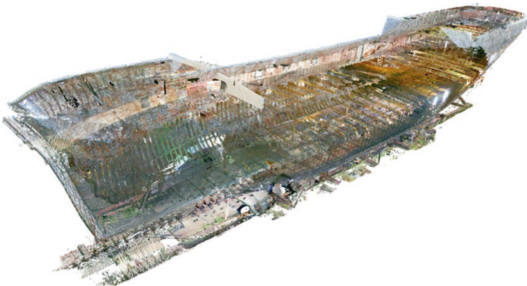
Fig. 7.2 Orthographic representation of the resultant point cloud acquired from the laser scan survey (Headland Archaeology Ltd.)
