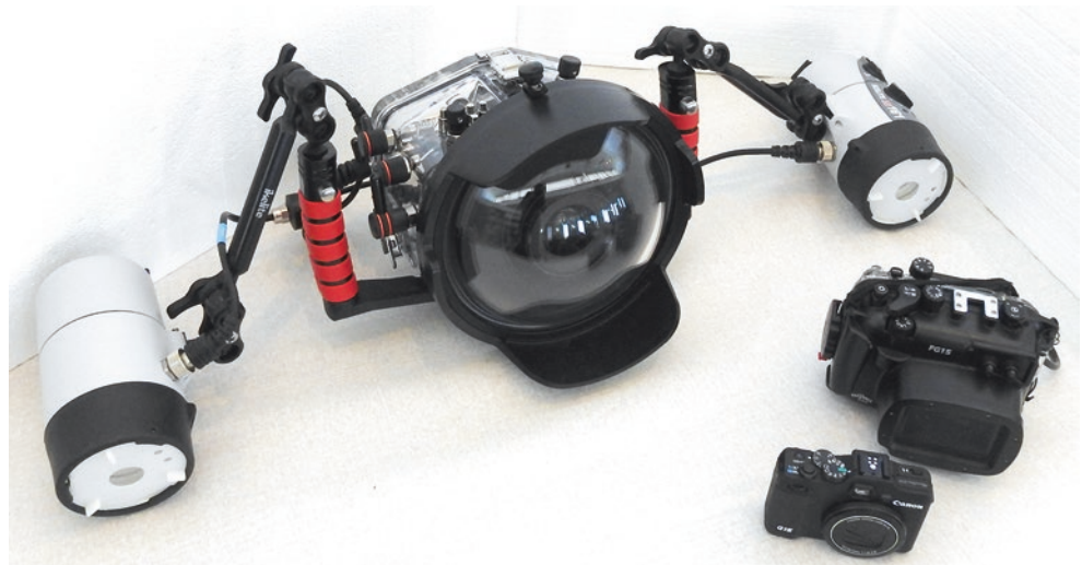
Fig. 5.7 Two of the camera systems used: to the left, the Canon EOS 70D DSRL with the Ikelite housing and to the right the Canon PowerShot G15 with the Fantasea housing (L. Semaan)
