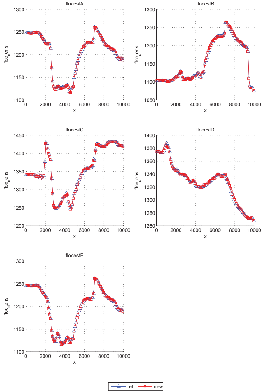
Figure 10.95: flocest : Horizontal profile of the surface floc mass density ( kg/m^3 ) along a mid-channel transect at the end of the simulation.
