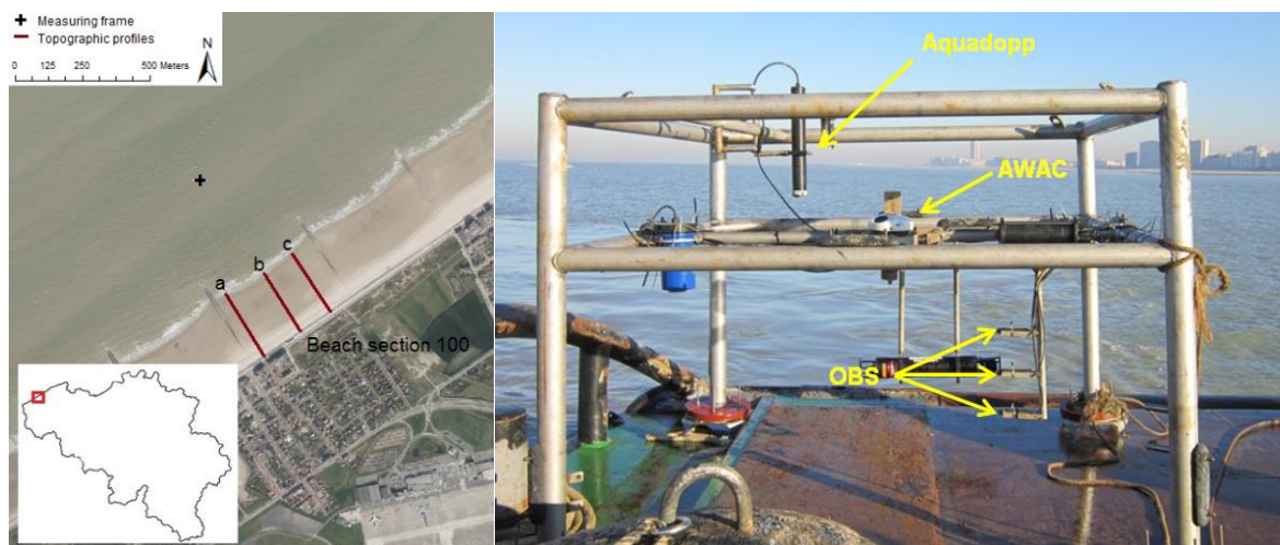
Figure 1. Study site and a picture of the measuring frame.
