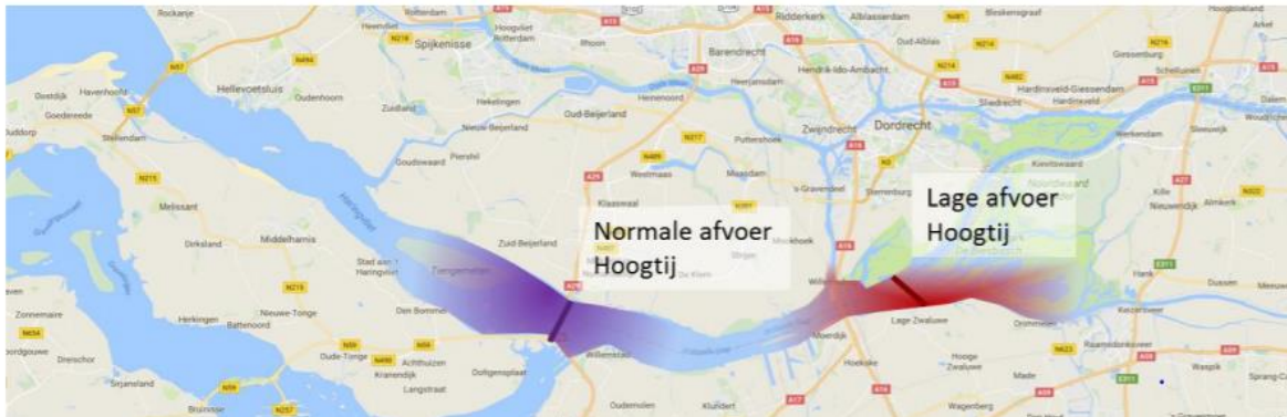
Figure 17 By modelling, the salt intrusion is determined in the Haringvliet during the scenario Stormvloedkering. The purple area indicates the salt intrusion during normal discharge and high tide, the red area indicates the salt intrusion during low discharge and high tide. The lines give the upper boundary of freshwater of 300 mg Cl per liter (salinity of 0.5 ppt) which will be the most likely, the purple and red area give the high uncertainties (Wijsman et al., 2018).
