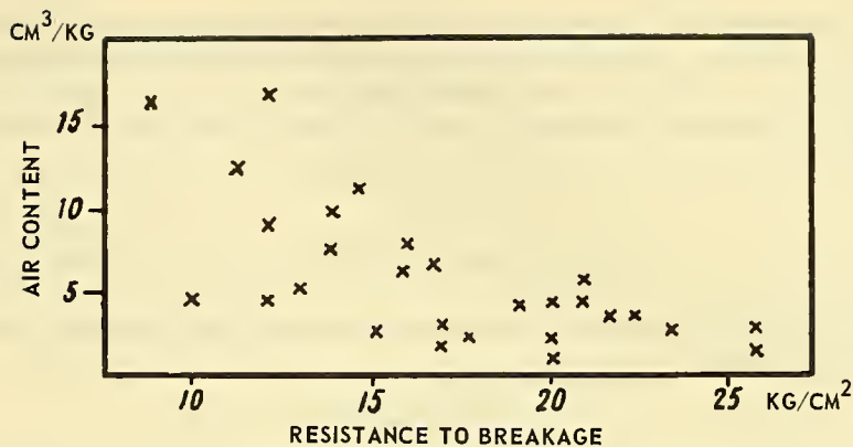
Figure 62. Limit of plasticity during breakage of ice with different air contents.
