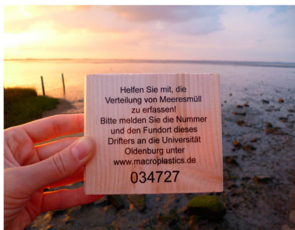
Figure 4.9.2. 1600 wooden drifters were released on 24.02.2018 and 27.02.2018 during the research cruise HE503 of the RV Heincke (Figure 4.9.1). (a) The wooden drifter (message in English is on the back side: 'Help us understand the distribution of marine litter! Please report the number and position of this drifter to the University of Oldenburg'). (b) Floating drifters after the deployment at Borkum Riffgrund.
