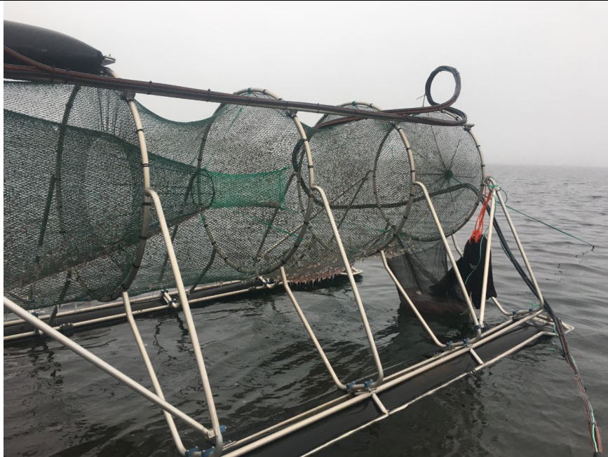
Alternative entrance in pontoon trap chamber. Traditionally strings are used in the chamber entrance. Also, the fish chamber is equipped with hose net for catch collection.
