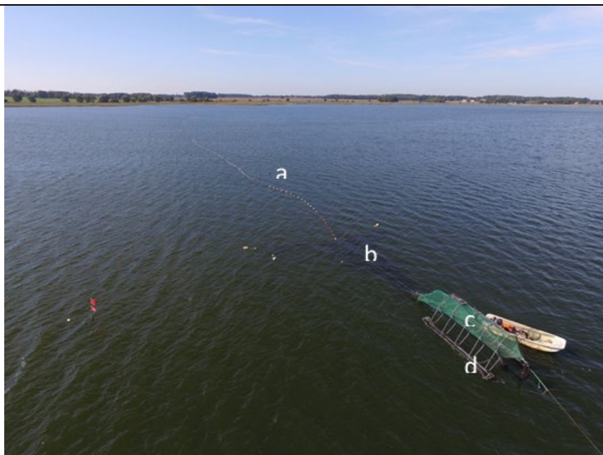
Stationary poundnet with pontoon trap catch chamber (arial view). a) guiding net; b) trapnet, c) catch chamber, d) pontoons
