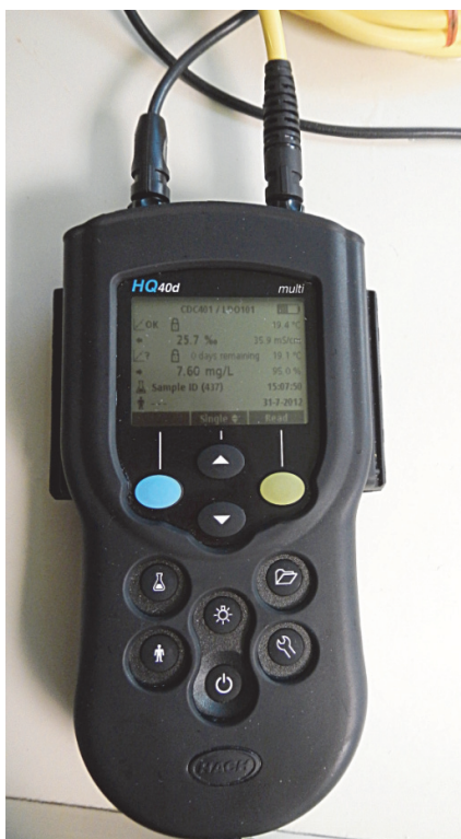
Figure 28 Hach HQ40d multimeter used for calibration/check of data from the PocketBox.
