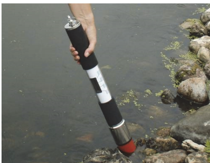
Figure 29 BenthosTorch measurement of a stone surface on a river bank (picture copied from http://www.bbe-moldaenke.de/chlorophyll/benthostorch/ )
