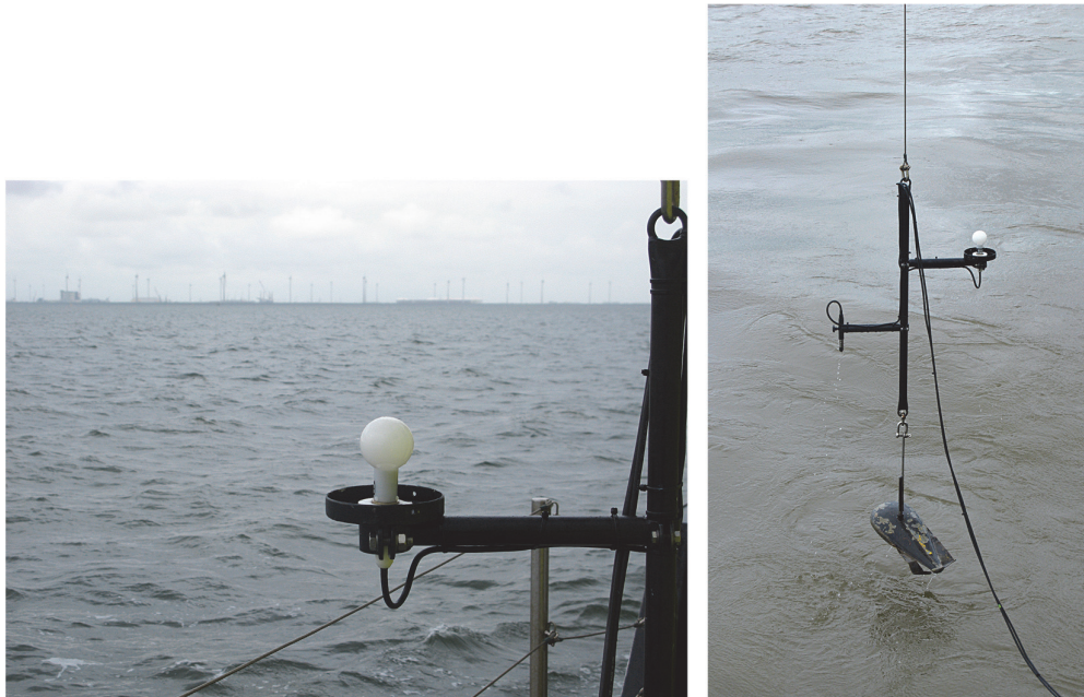
Figure 39 The LICOR light sensor that was lowered under water to construct a light attenuation profile under water at each sampling station. A similar sensor was kept on deck to store actual incident radiation.
