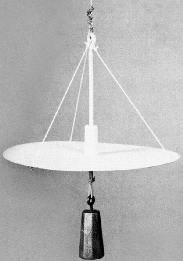
FIGURE 1. Luksch's polished white painted Secchi disk, 45 cm in diameter, was used onboard the vessel Pola .
