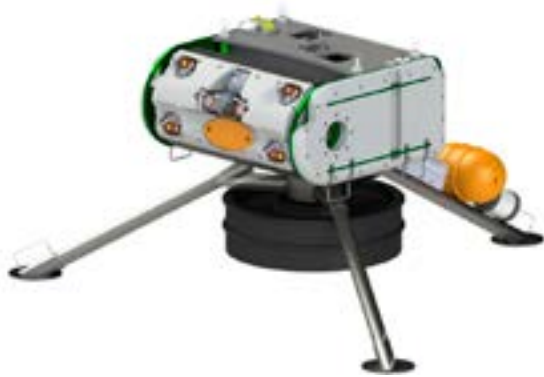
Figure 10.10. The Adaptable Monitoring Package (AMP). An integrated subsea instrument package developed by the University of Washington that is used to monitor MRE devices. (Image courtesy of Applied Physics Laboratory, University of Washington)
