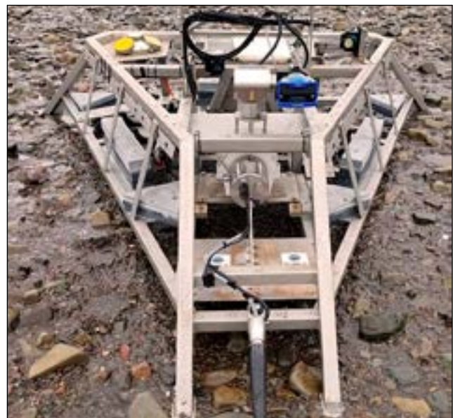
Figure 10.11. FORCE's Fundy Advanced Sensor Technology Environmental Monitoring System (FAST-EMS) integrated and cabled monitoring platform positioned on the FORCE beach. (Photo courtesy of FORCE)
