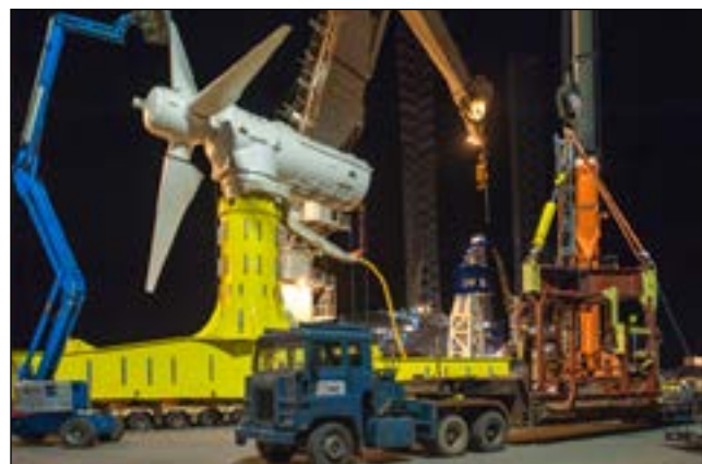
Figure 3.1. A MeyGen tidal turbine ready for deployment in the Inner Sound of Pentland Firth in Scotland. (Photo courtesy of SIMEC Atlantis Energy)
