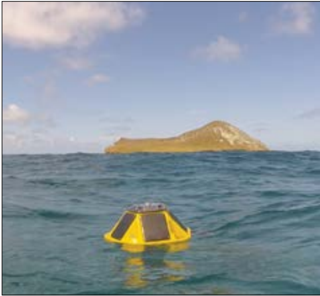
Figure 7.4. Spotter (Sofar Ocean) real-time wave measurement buoy. (Photo courtesy of Grace Chang)
