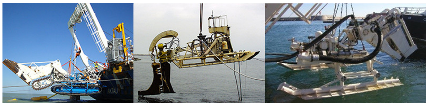
Fig. 1. Wheel cutter (left); Plough (centre) and Towed Jetting Vehicle (right) (courtesy: www.ldravocean.com).
