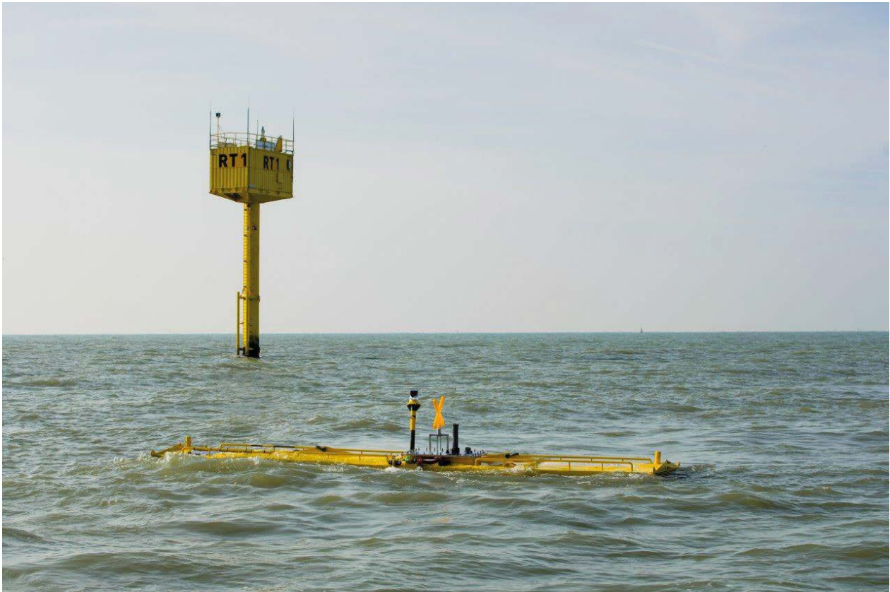
Figure 4. The NEMOS Wave Energy Converter prototype at the site of the Blue Accelerator (photo NEMOS).
