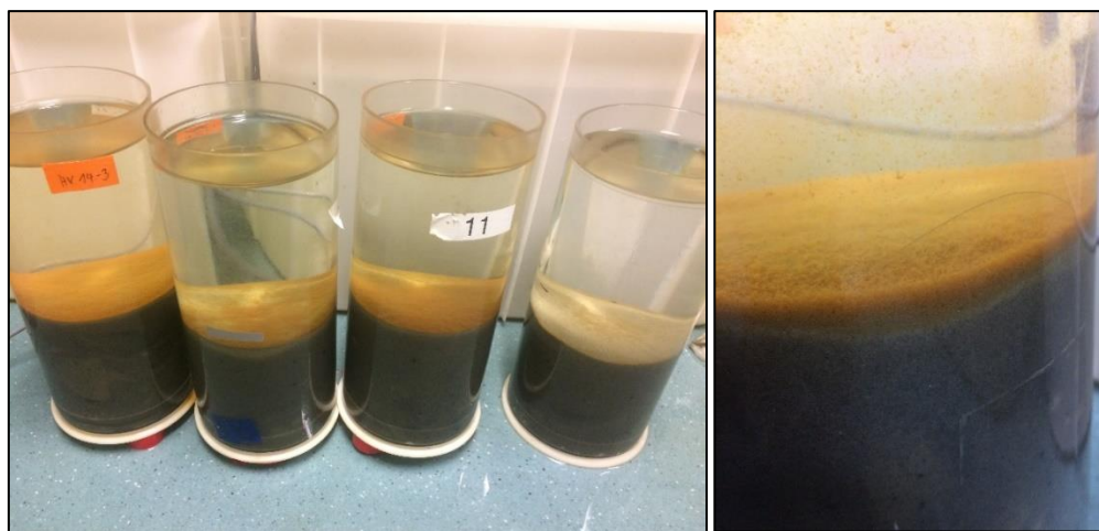
Figure 8. Photos of iron oxide formation in three PDC exposed cores next to one control core (left). A closer look at newly formed iron oxides on the sediment surface and in the water column (right).
