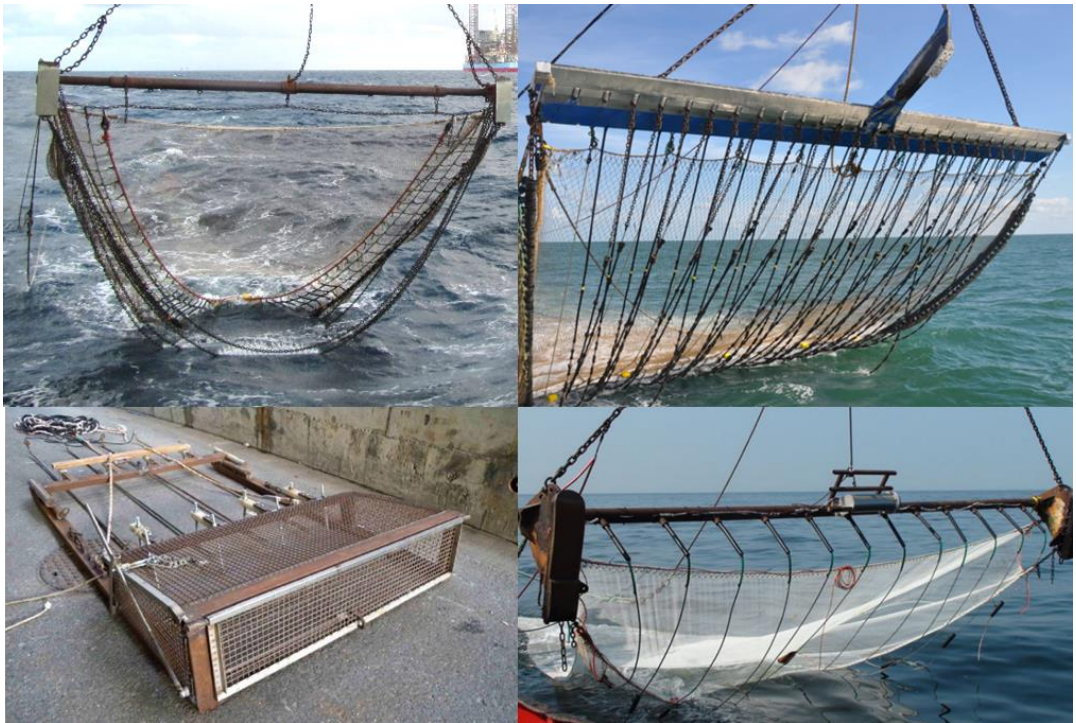
Figure 2. Comparison between a traditional tickler chain rigged beam trawl (top left) and an electric PulseWing trawl (top right) which are both used to fish for North Sea dover sole ( Solea solea ). Electrodes and gear used to stimulate and catch razor clams, Ensis spp. (bottom left) and a ‘Hovercran’ electric trawler used to catch brown shrimp, Crangon crangon (bottom right).
