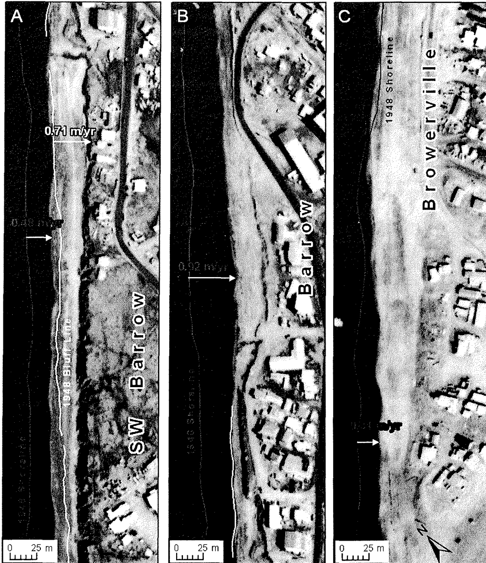
Figure 2. Coastal strips of the 1997 orthophoto mosaic, showing the position of the 1948 shoreline and bluff line. Also shown are shoreline and bluff-line erosion rates for selected areas.
