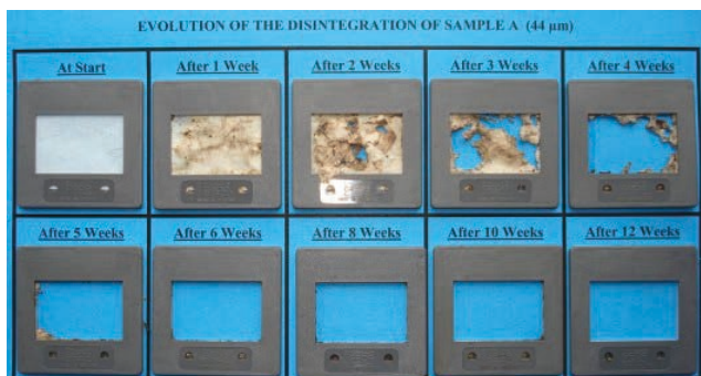
Figure: Example of disintegration test (source OWS).
