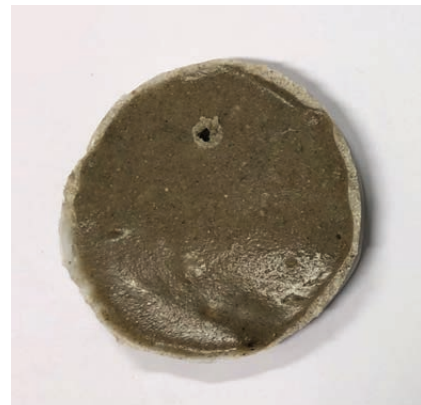
Figure: Small scale tests have shown that the concept of a temporary, biobased and biodegradable gravity anchor works; after 3 months in seawater at 22°C we observed 7-9% weight reduction of the sample. On the sample one observes clear growth of microorganisms.
