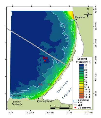
**Figure 8.** Probability of ice cover observations (%) in the SE Baltic near the Curonian Spit in February according to spaceborne SAR data during an extended period of 2004–2019 [14]. Light blue contours show isolines of 2% and 5% probabilities of ice cover observations.
