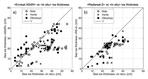
**Figure 11.** Scatter plots of in-situ ice thickness measurements made at Nida, Ventė and Otkrytoye stations versus (**a**) Envisat ASAR 0.5-km and (**b**) RADARSAT-2 0.5-km ice thickness products.
