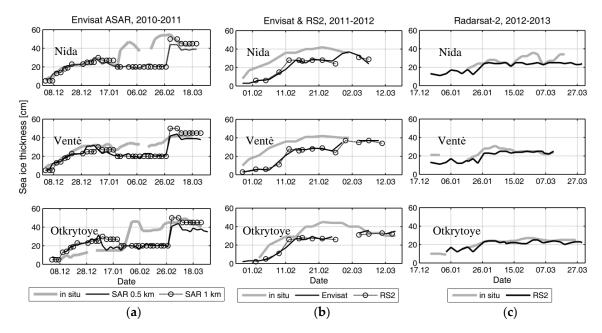
**Figure 10.** Comparison of Envisat ASAR and RADARSAT-2 ice thickness products with in-situ measurements for winter seasons of 2010–2013 for (a) Envisat ASAR 0.5-km and 1-km products in 2010–2011, (b) Envisat ASAR 0.5-km and RADARSAT-2 0.5-km products in 2011–2012, (c) RADARSAT-2 0.5-km in 2012–2013.
