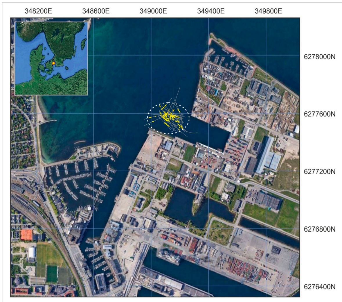
Figure 17. Map of the acoustic anomaly in Svanemøllen Harbour, Copenhagen, Denmark. The sailing lines are grey, the response features (haystacks and narrow noise columns) are yellow. Zone 33 UTM coordinates. Graphics: Grøn.
