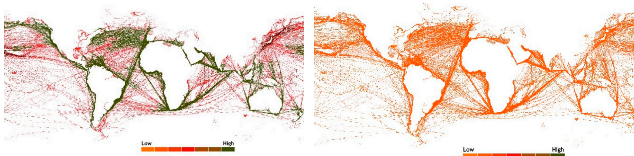
Figure 4. Annual global container shipping SO x emission levels for 2020, (left) base situation for 2018 and (right) estimates using the energy consumption approach, based on extrapolated data from IHS Markit Portal [2].
