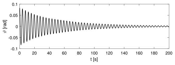
Figure 8. Free decay test for the inverted spring-damper pendulum.
