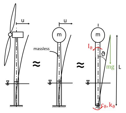
Figure 2. Equivalent monopile model.
