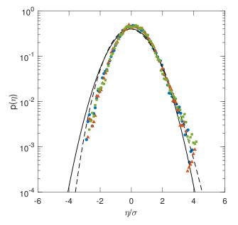
**Figure 10.** Probability density function of the surface elevations with respect to the surface elevations normalized by their standard deviation, as computed by near-field time domain for BFI = 0.09 (•), BFI = 0.58 ( $\blacktriangle$ ) and BFI = 0.73 ( $\blacksquare$ ) plotted against the normal pdf (full line) and its second-order correction (dashed line).
