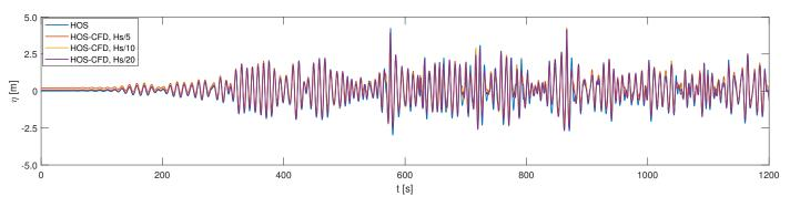
**Figure 5.** Benchmark with surface elevation plotted against time for the higher-order spectral (HOS) model (blue) and the coupled model for mesh resolutions Hs/5 (red), Hs/10 (yellow) and Hs/20 (purple).
