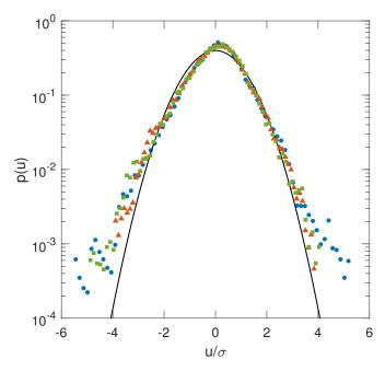
**Figure 12.** Probability density function tower top displacements with respect to the displacements normalized by their standard deviations, as computed by near-field time domain for BFI = 0.09 (•), BFI = 0.58 (▲) and BFI = 0.73 (■) plotted against the normal pdf (–).
