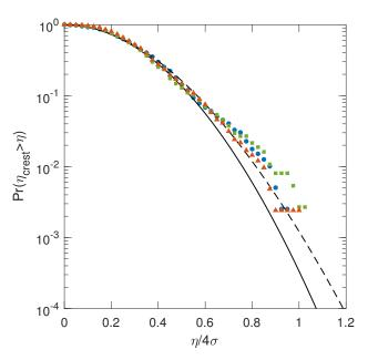
**Figure 11.** Probability distribution of the wave crests with respect to the wave elevations normalized by their standard deviations, as computed by near-field time domain for BFI = 0.09 (•), BFI = 0.58 (▲) and BFI = 0.73 (■) plotted against the Rayleigh distribution (full line) and the Tayfun distribution (dashed line).
