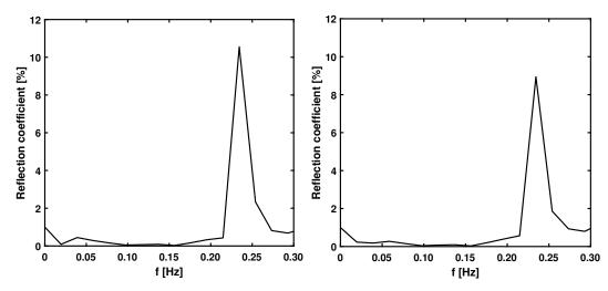
Figure 7. Reflection coefficients for higher-order spectral numerical wave tank (HOS-NWT) (left) and OpenFOAM (right).
