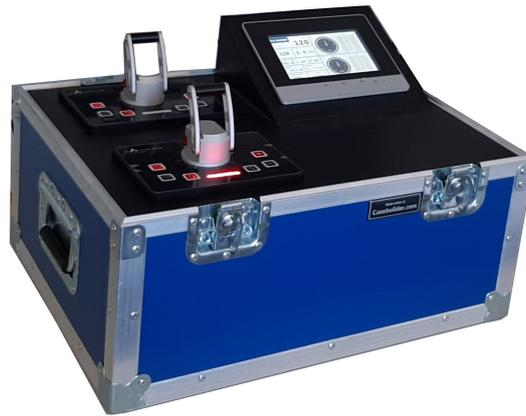
**Figure 8.** The I-SCC motion control subsystem: two azimuth controllers on the left and a touch screen on the right.
