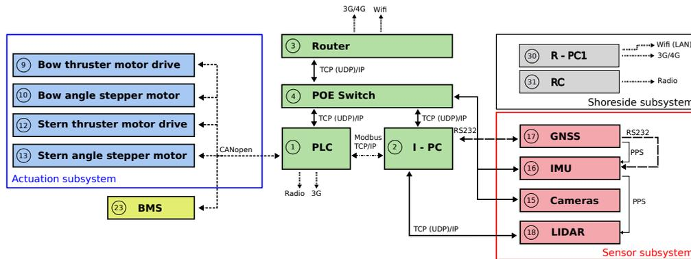
**Figure 3.** Main USV system components and their communication links, adapted from [5] with permission from Elsevier, 2020.
