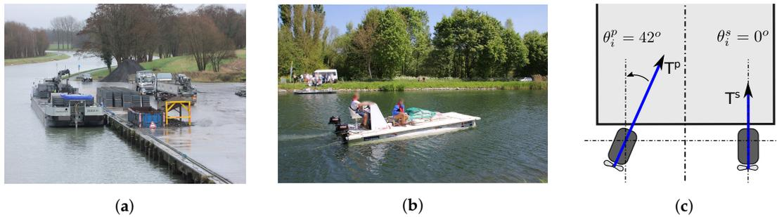
**Figure 4.** The pallet shuttle barge: (a) a real barge’s handling cargo at a dock [40], (b) the KU Leuven scale model named Maverick, and (c) the propulsion system of Maverick consisting of two outboard motors which can rotate between  $[-42, 42]^\circ$  and which can have different thrust force magnitudes.
