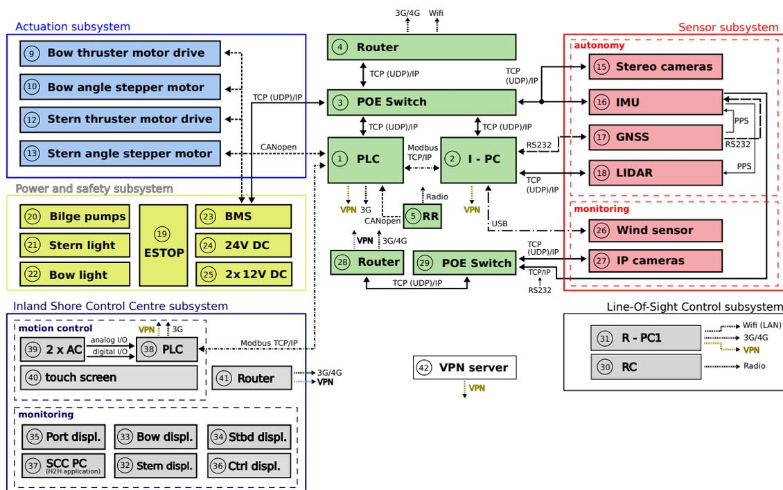
Figure 7. Main I-SCC and USV components and their communication links.
