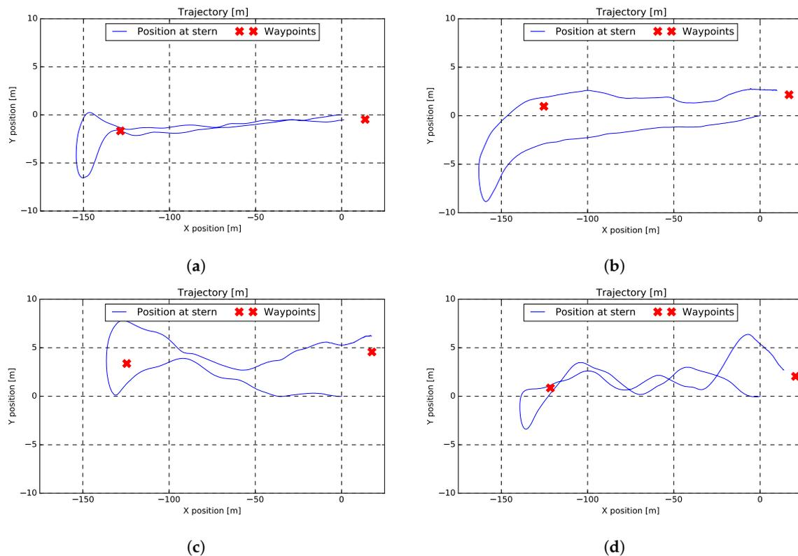
**Figure 16.** H2H-extended I-SCC straight sailing experiment with the USV in a canal (Leuven): (a) participant one, first run, with H2H-application  $\approx 8.5$  min, (b) participant one, second run, without H2H-application  $\approx 10$  min, (c) participant two first run, without H2H-application  $\approx 7$  min, and (d) participant two, second run, with H2H-application  $\approx 6$  min.
