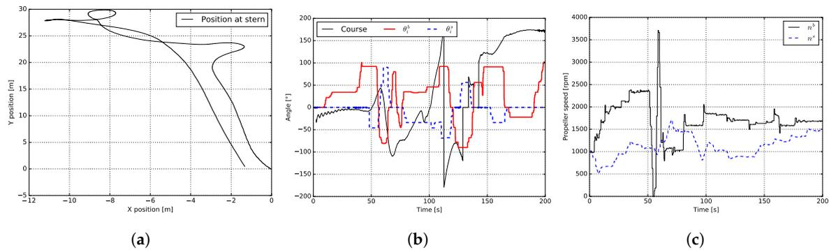
**Figure 13.** USV under I-SCC motion control in a canal (Leuven): (a) sailed trajectory, (b) internal actuation angles and USV course, and (c) actuation rotational speeds.
