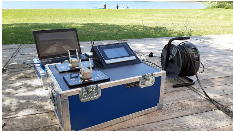
**Figure 18.** Moveable motion control subsystem of the I-SCC system, deployed at Rotselaar lake.
