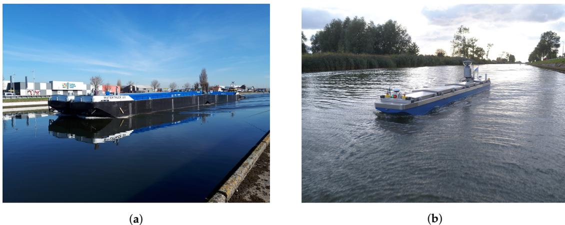
**Figure 1.** The Watertruck<sup>+</sup> concept [32]: (a) four real-size barges pushed by a push boat, reproduced from [5] with permission from Elsevier, 2020, (b) the KU Leuven scale model of a self-propelled barge named Cogge [5].
