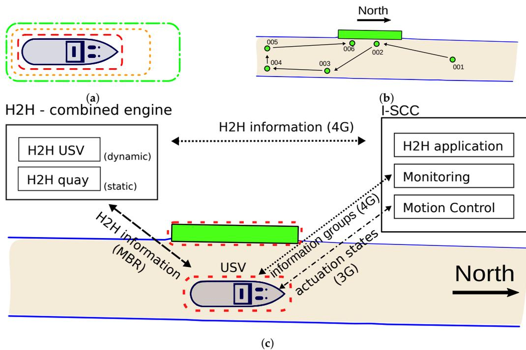
**Figure 6.** Augmented remote motion control and monitoring within the H2H project: (a) proximity zones, (b) envisaged design docking manoeuvre experiments, and (c) design philosophy of the H2H-extensions on the I-SCC design.
