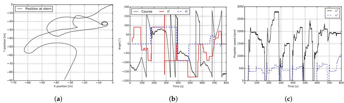
**Figure 14.** USV under I-SCC motion control in a lake (Rotselaar): (a) sailed trajectory, (b) internal actuation angles and USV course, and (c) actuation rotational speeds.
