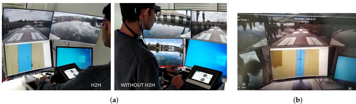
**Figure 17.** Single-handed sailing with the USV and I-SCC system on a canal (Leuven): (a) Video S2: docking manoeuvres from a participant (left) with the H2H-application, and (right) without the H2H application; (b) Video S3: tracking of the eye movements of a participant during the 180° turn of a straight sailing experiment.
