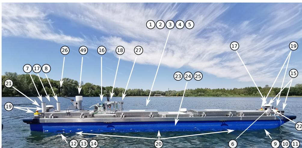
**Figure 10.** Positions of the main onboard USV components, referring to Table A1. Note that the LIDAR (number 18) was not mounted, but can be seen in Figure 1b.
