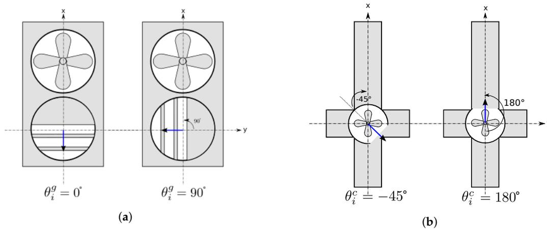
**Figure 2.** An abstract bottom section of the nested 360-degree-steerable actuators, where the x-axis points to the bow, the y-axis starboard, and the z-axis downwards. The blue arrows denote the theoretical orientation of the water exiting the systems: (a) steering-grid thruster placed at the bow, and (b) four-channel thruster positioned at the stern, adapted from [39] with permission from MDPI, 2020.
