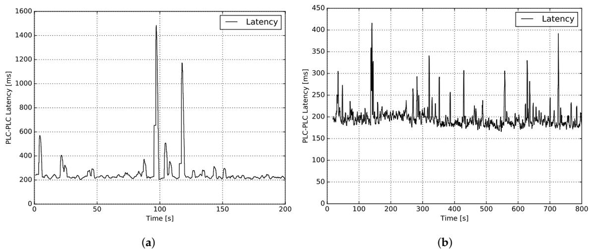
**Figure 15.** Latency time between onboard and onshore PLCs: (a) canal in Leuven, and (b) lake in Rotselaar.
