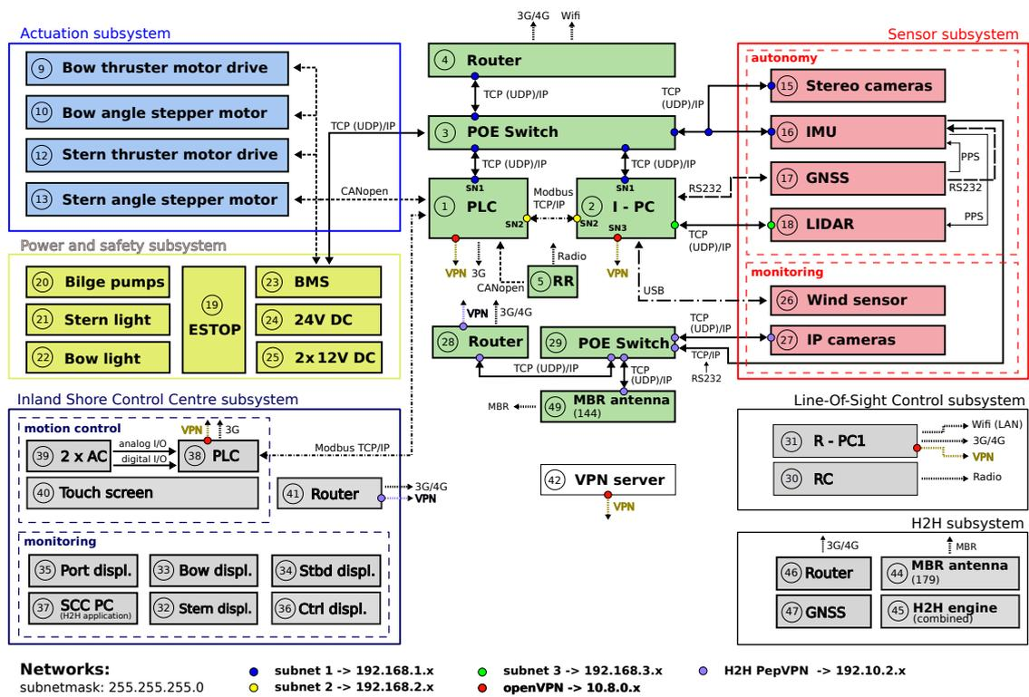
Figure 11. H2H-extended I-SCC and USV system design: main components and their communication links.
