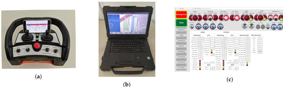
**Figure 5.** The previous line-of-sight shore side control components (summer 2019): (a) wearable remote controller with web-interface, (b) the rugged computer (R-PC) running MOOS-IvP, and (c) an additional laptop monitoring the PLC web-interface.
