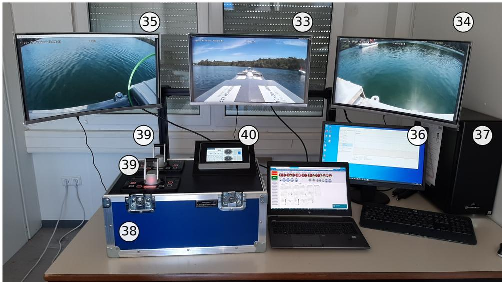
**Figure 9.** Constructed I-SCC streaming video data from the USV sailing on the Rotselaar lake (see Section 5.1), part numbers refer to Table A1.
