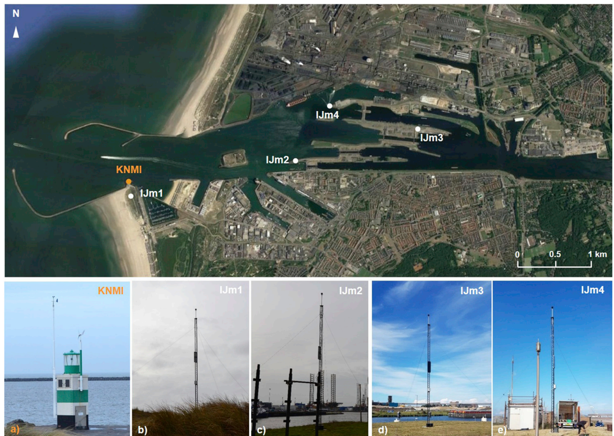
Fig. 5. Positions of the 2D ultrasonic anemometers installed in the IJmuiden sea lock. Also the anemometer station of the Royal Dutch Meteorological Institute (KNMI) is shown. Top view photo credit to Google Maps.
