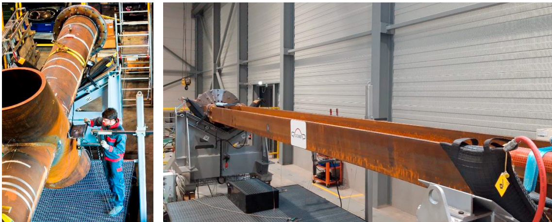
Figure 2: welded X-joint node (left) and beam (right) in the CRONOS test setup.
