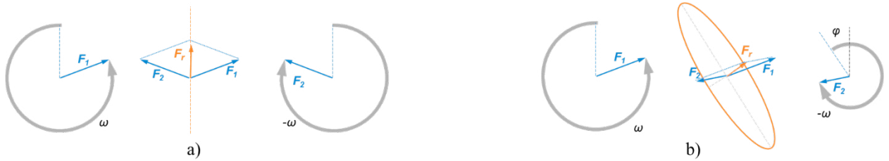
Figure 3: Combined force vectors for the double excenter assembly: a) F_1 = F_2 ; b) F_1 > F_2 .
