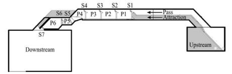
Fig. 1. Fish pass layout (scale model version: P5 is shortened compared to prototype).
