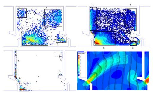
Fig. 3. Pool P1, Presence areas: (a) bleak; (b) chub; and (c) bullhead. (d) Computed flow pattern, velocity from 0 to 3 m/s [4].
