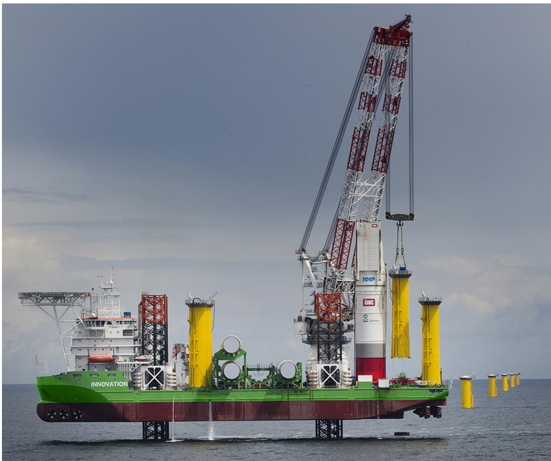
Figure 1: The offshore heavy lift DP2 jack-up vessel Innovation (DEME group).
