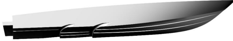
Figure 1: Double stepped hull - side view.
