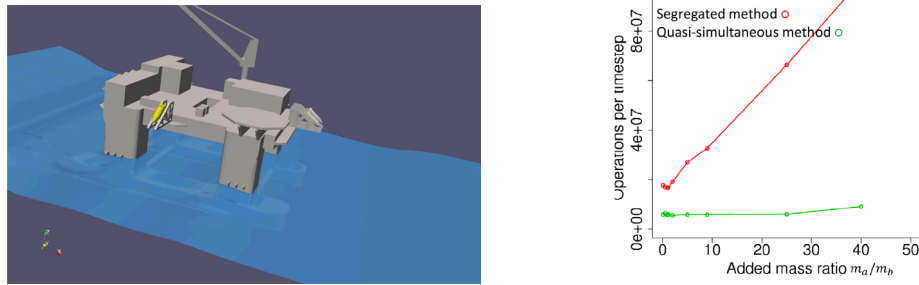
Figure 5: Free-fall life boat being launched (left). The computational effort required per time step for the FSI coupling (right).
