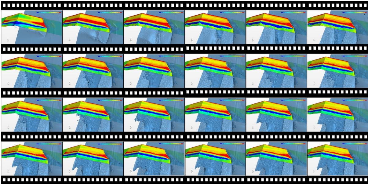
Figure 5: Flow field snapshots of N-S simulations at \sigma_0 = 2.35 . Bottom view (on foil face). Frame sampling rate: first row \Delta t=2.4 ms, second row \Delta t=4.8 ms, third/fourth rows \Delta t=9.6 ms. Color contours indicate pressure coefficient, air/water free surface rendered in transparent blue (on left side of V-hydrofoil only).
