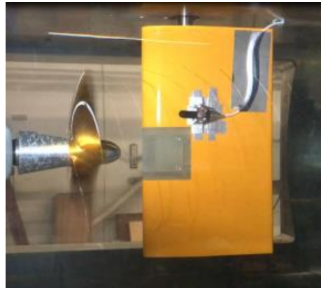
Figure 8: The arrangement of cavitation noise measurement
