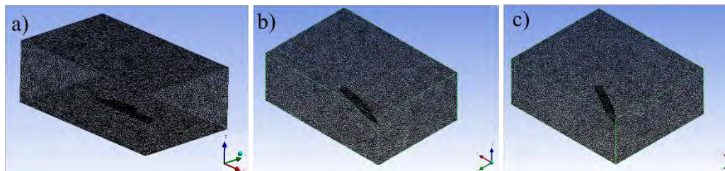
Figure 3: Mesh generated for 0^\circ, 15^\circ and 30^\circ (a, b, c) cases in ANSYS Mesh Generator.
