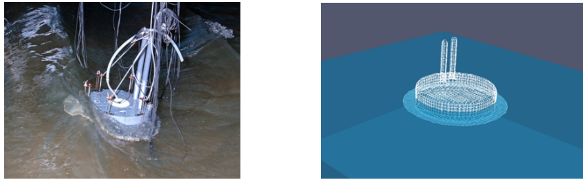
Figure 6: Model of the CALM buoy in the shallow water basin at MARIN (left) and the geometrical representation in the simulations (right).
