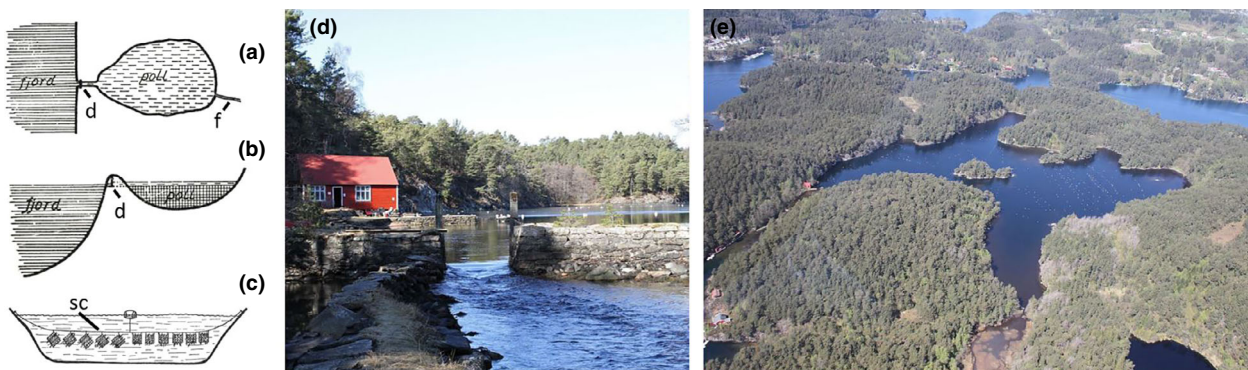
Figure 6 Breed polls schematics and illustrations of a breed poll: (a) view from above of a breed poll and connectivity to the Fjord, (d) drain that can be closed, (f) inlet of freshwater; (b) profile view of a breed poll and connectivity to the fjord, (d) drain that can be closed; (c) schematic of the method for hanging seed collectors, (sc) suspended seed collectors; (d) view of the dam of the Innerøy Poll in Norway; (e) aerial view of the Innerøy Poll. Modified after Gaarder and Bjerkkan (1934) and photographs from KVB and Anonymous (2017).
