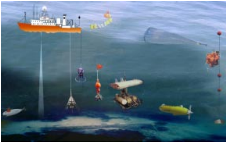
Fig. 40. Equipment used for exploring the oceans. (Top: a research ship towing an array of sensors and a net near the surface; Left to right: remotely operated vehicle, a sound pulse to measure depth, multiple sampler for sea floor sediments, conductivity - temperature - depth sensor with water samplers, boomerang grab for manganese nodules, underwater video and photo system, autonomous underwater vehicle, deep-sea mooring for deploying current meters and sediment traps for long duration of time).
