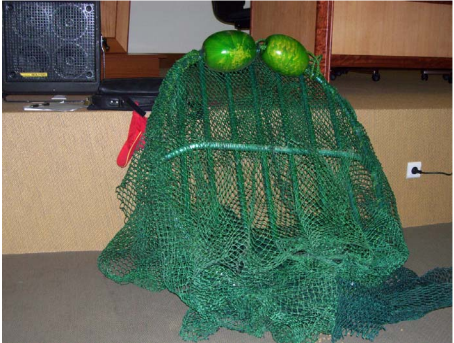
Plate 1. TED grid fixed in Codend Extension
