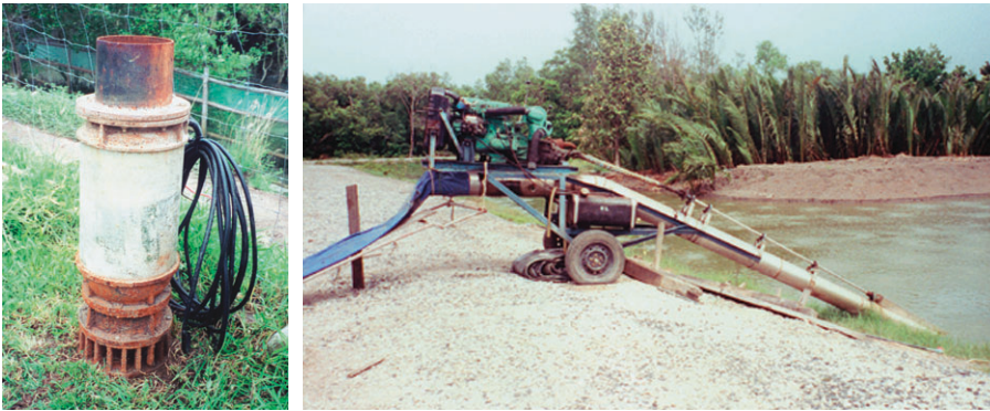
Fig. 13. Electrical water pump and diesel-powered water pump.
