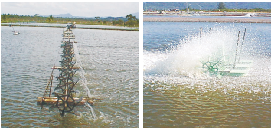
Fig. 11. Types of aerators commonly used in shrimp farms in Thailand and now being used in the Philippines.
