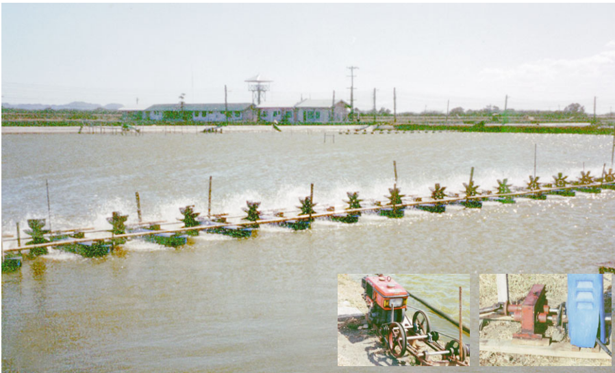
Fig. 10. Long-arm paddlewheel aerator. Inset shows the diesel engine (8hp) and electric motor (1hp), connected to a speed reducer designed to operate long arm paddlewheel with 10 to 15 empellers.
