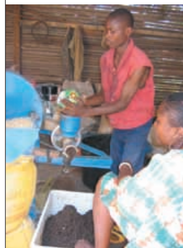
FIGURE 1 Adapted equipment for the production of fish pellets in Fouban, Cameroon
