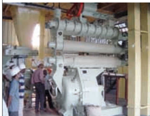
FIGURE 9 Shrimp pellet mill with triple-pass conditioning
