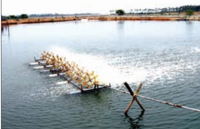
FIGURE 5 Indigenous aerator used in a shrimp culture pond
