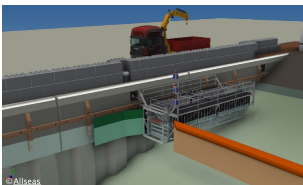
Figure 20 : 'Patje Plastic' the Port of Antwerp's plastic catcher installed at Doel dock
