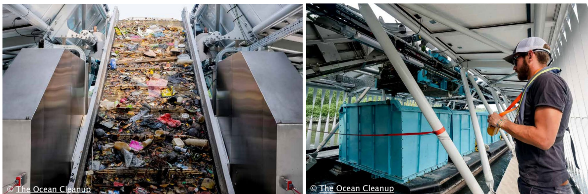
Figure 7 : Close up of a Conveyor belt system used to collect the plastic from the water (left) and the barge containers for easy transport and exchange of containers (right).
