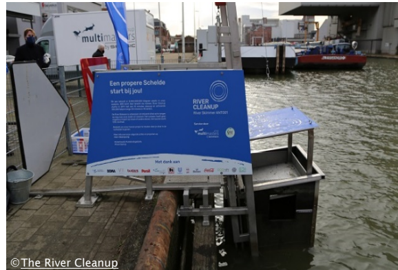
Figure 21 : The River cleanup initiative's River Skimmer installed at Oostkaai in Merksem
