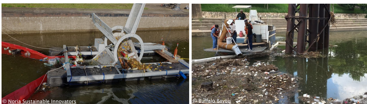
Figure 8 : Examples of alternative techniques to remove the plastic from the water: a waterwheel (Noria's CirCleaner) and a vacuum cleaning device (Buffalo Bayou's Bio-Vac).
