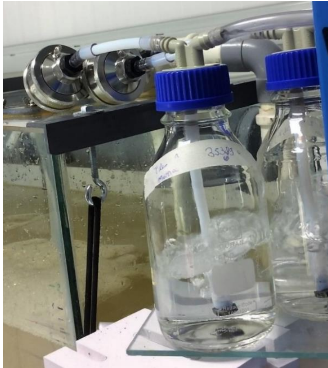
Figure S3.17: The additional SSA sampling technique used in natural and artificial seawater MART experiments to control the collection efficiency. The air passing through the quartz filters was drawn (in small bubbles) through pure water following the sampling method described by Tsunogai et al. 201
