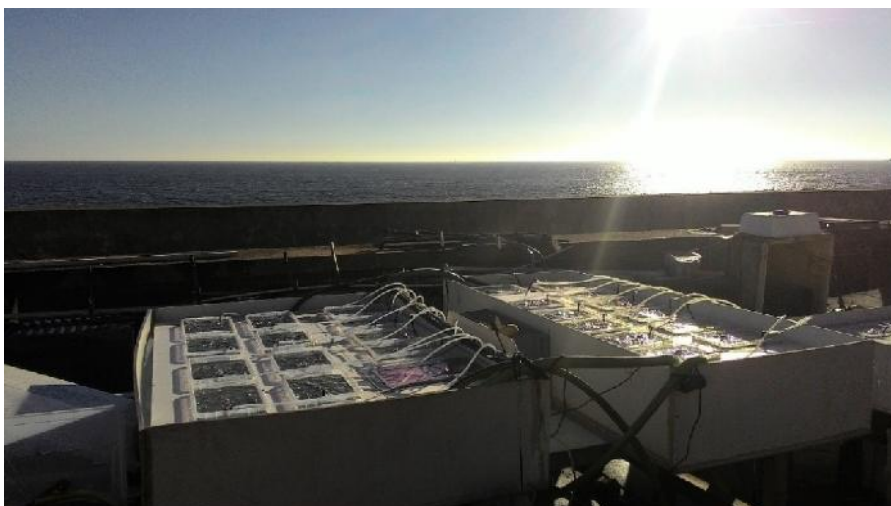
Figure Chapter IV Overview of an outdoor mesocosm experiment where seawater temperature and nutrient availability are manipulated to assess the physiological responses on the kelp Laminaria ochroleuca . Photograph by J.N. Franco
