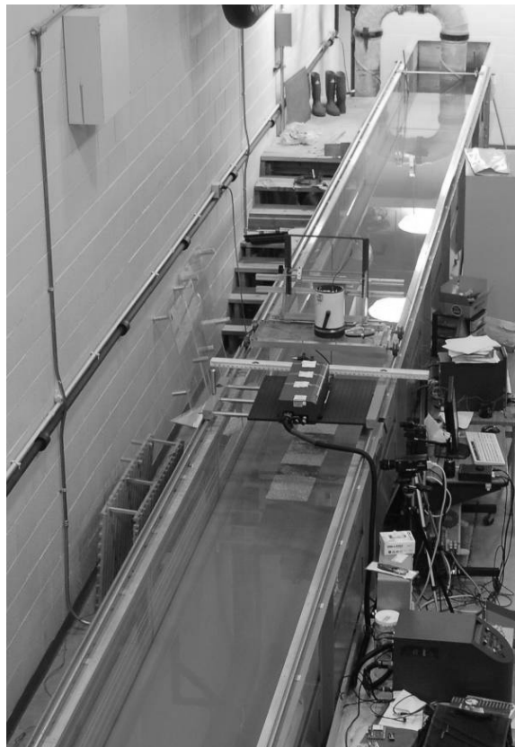
Figure 10. Test section of open channel flume at UWM hydraulic lab.
