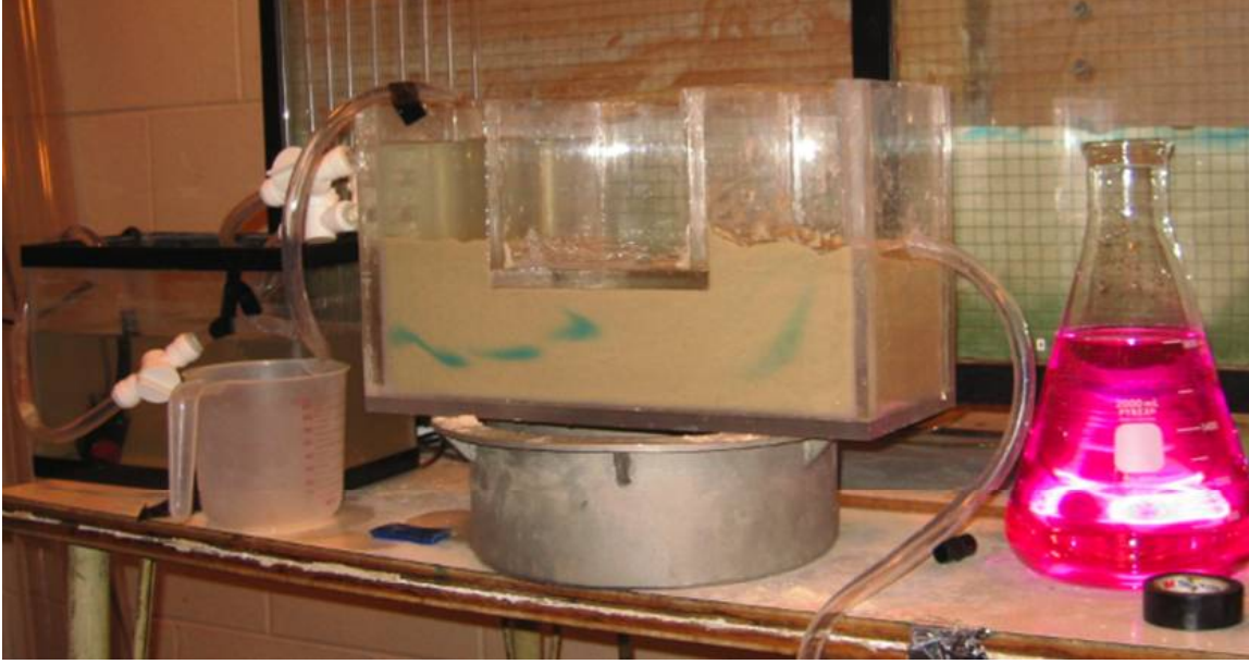
Figure 20. Dye tracing in the pore-water flow tank.
