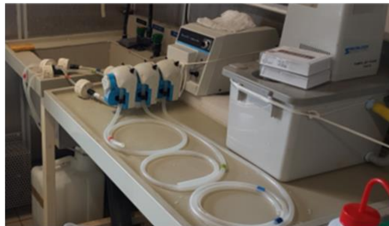
Fig. 4.3 | Upper panel (A). Left: filtration structure with 25 L containers and 200 \mu\text{m} and 20 \mu\text{m} filtration meshes. Mid: filtration set-up for 142 mm filters with a peristaltic pump and filtration tripods (3 \mu\text{m} and 0.22 \mu\text{m} ) and filter cutting tray. Right: Filtration tripod 3 \mu\text{m} in detail. Lower panel (B) In-line filtration set-up for 47 mm filters with a peristaltic pump.
