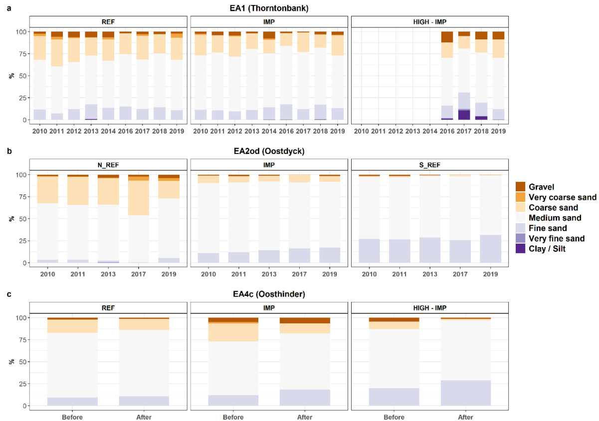
Figure 5: Relative sediment composition (%) for the three EAs for each impact group, i.e. REFERENCE, IMPact, HIGH-IMPact, N_REF and S_REFERENCE samples (the latter respectively north and south of the extraction hotspot in EA2od). For EA1 (Thorntonbank) and EA2od (Oostdyck) sampled years are shown, while for EA4c (Oosthinder) 'before' and 'after' extraction periods are shown. Legenda: Gravel >1600 \mu\text{m} , Very coarse sand 1600 - 1000 \mu\text{m} , Coarse sand 1000 - 500 \mu\text{m} , Medium sand 500 - 250 \mu\text{m} , Fine sand 250 - 125 \mu\text{m} , Very fine sand 125 - 63 \mu\text{m} , Clay to silt 63 - 0 \mu\text{m} .
