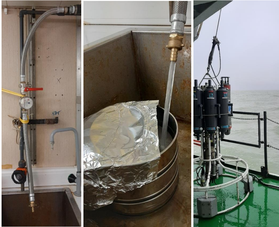
Figure 3.2: Water sampling. Left: Seawater inlet pump equipped with a flowmeter. Middle: water filtration from the inlet through metal sieves (100µm, 63µm), covered with aluminium foil to prevent air contamination. Right: Rosette with the 5l Niskin bottles.
