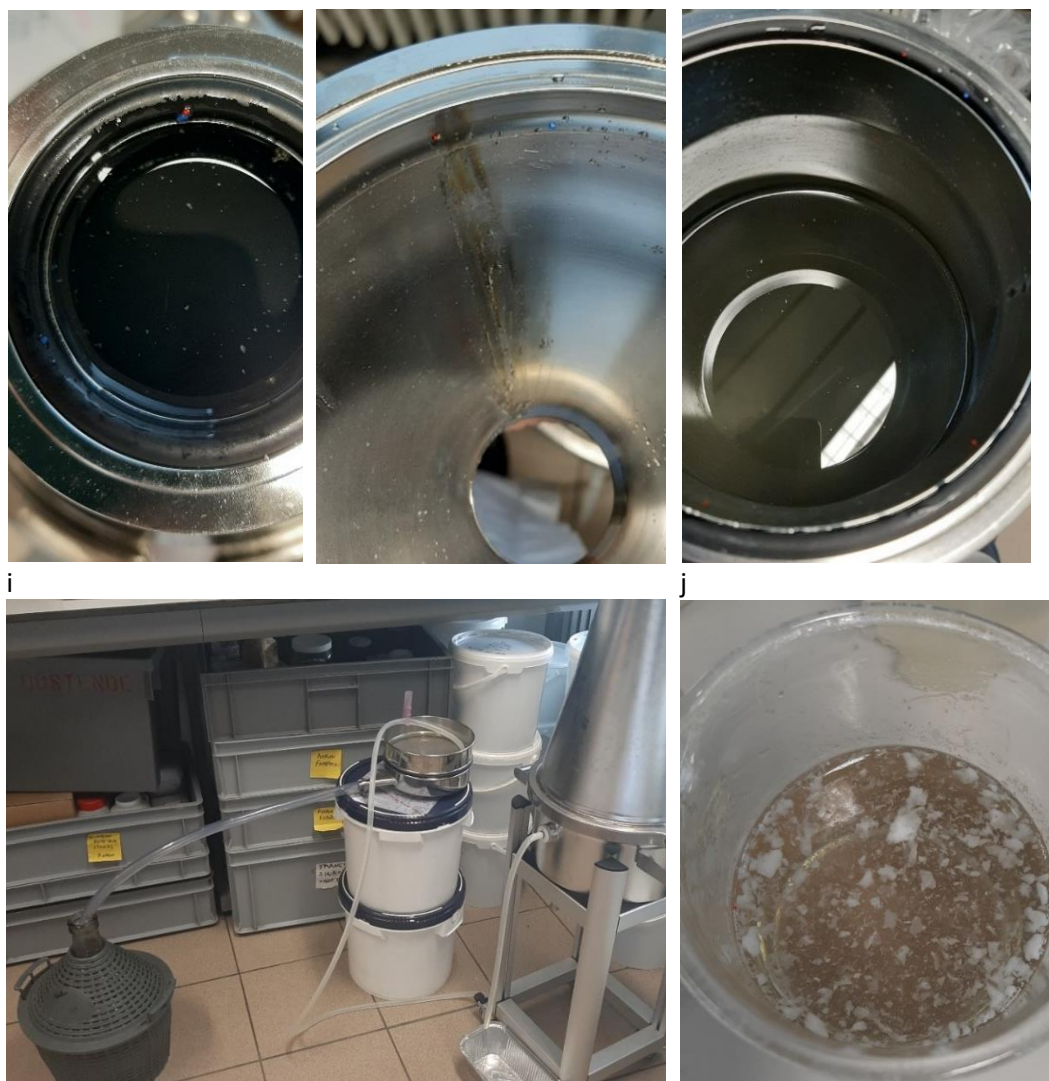
Figure 3.4: a-b: Components of the MPSS; c-d: Slight leakage from the ball valve; e: Foam in the sample chamber; f-h: Spikes (blue and red) stuck on different MPSS parts; i: Cleaning of the density solution (20 \mu m sieve) before storage in glass jars; j: Reaction of NaBr + SDS (1%) =white precipitate
