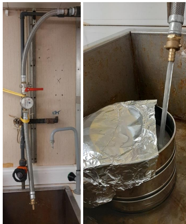
Figure 1: Water sampling. Left: Seawater inlet equipped with a flowmeter. Right: water filtration from the inlet through metal sieves (100µm, 63µm), covered with aluminium foil to minimise air contamination.
