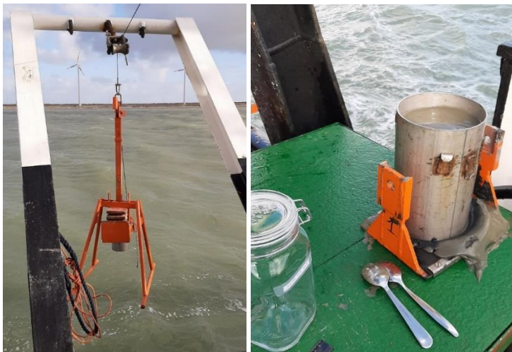
Figure 3.3: Sampling with Reineck box corer
