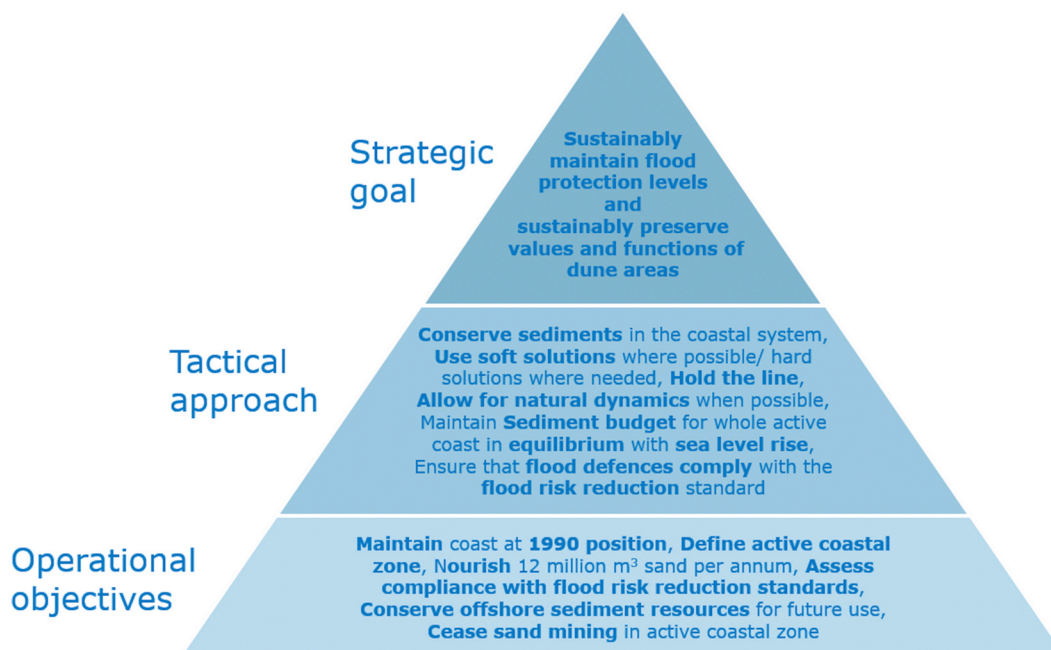
Fig. 3. Strategic goal, tactical approach and operational objectives of the current dynamic conservation policy (adapted from Lodder et al., 2019).
