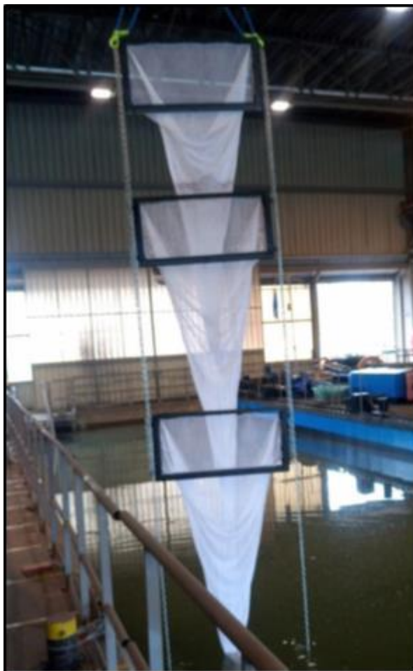
Fig. B.2. Suspension sampler used to perform observations at different depths in the water column
