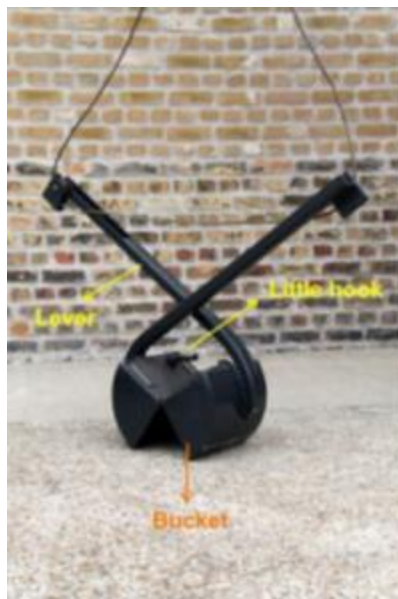
Fig. B.4 A Van Veen grab is a simple instrument to collect sediment samples
