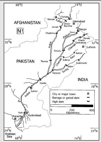
Figure 4. Map of the Indus river system in Pakistan showing barrage and high dam projects (planned, underway, and already constructed).
