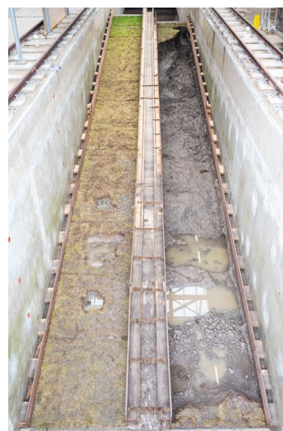
Figure 2: Erosion profile in the “Deltagoot” (Deltares) (P. van Steijn, M. Klein Breteler; 2021)
