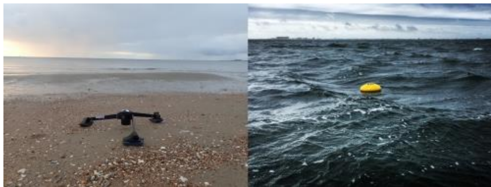
Figure 1: The Nortek Eco deployed at the field site using its tripod bottom mount and buoy system.
