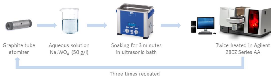
Figure 1 Scheme of graphite furnace surface-modification
