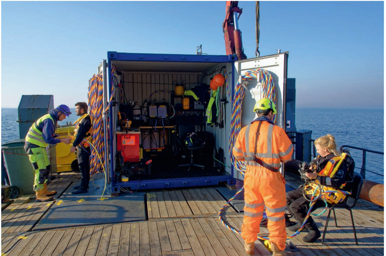
Fig. 6: Dive container setup for an archaeological offshore diving project. The standby diver is being checked by the supervisor, while the main diver is being dressed by the tender. © LaKD M-V, Landesarchäologie, Auer 2018
