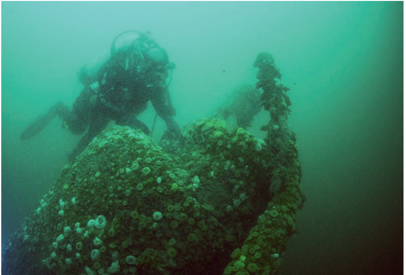
Fig. 2: Conning tower of UB-29, with one visibly bent periscope. © Termote & Mouchart
