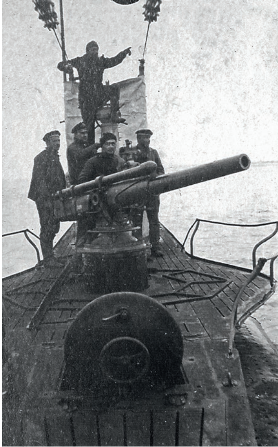
Fig. 9: Crewmen stand ready around the 8,8 cm deckgun of a UB-II type submarine. © Termote
