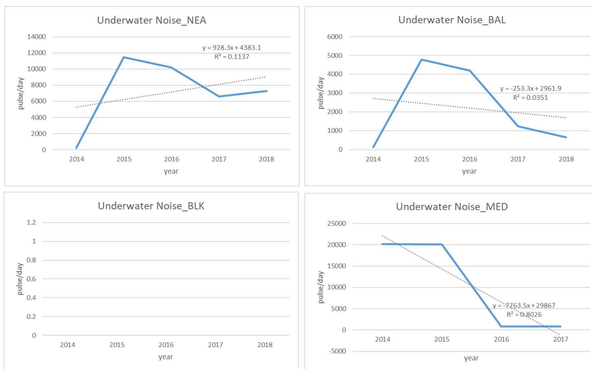
Figure 1. Underwater impulsive noise and relative trend in the European marine regions: North-East Atlantic (NEA), Baltic Sea (BAL), Mediterranean Sea (MED) and Black Sea (BLK). Time-series indicator: underwater noise, 2014-2018.
