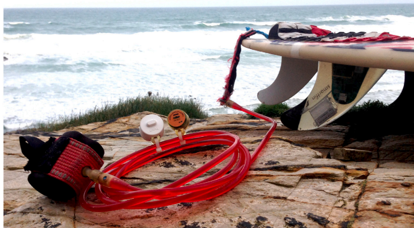
Fig. 1. Photo of equipment used by surfers to measure water temperature. Tidbit sensors (shaded (white) and unshaded sensor) on leash of surfboard, and Smartfin, with integrated environmental sensor package (surfboard fin closest to the leash). Detailed descriptions of the system are provided by Brewin et al. (2015, 2017b, 2020b) .
