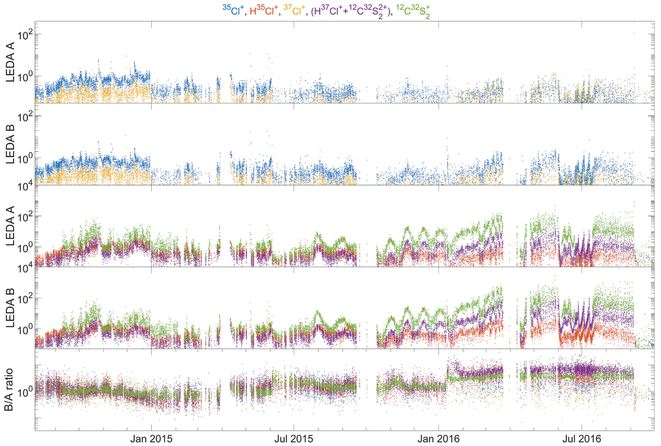
Figure 2. Ion counts per second ( R_Y ) for ^{35}\text{Cl}^+ , \text{H}^{35}\text{Cl}^+ , ^{37}\text{Cl}^+ , (\text{H}^{37}\text{Cl}^+ + ^{12}\text{C}^{32}\text{S}_2^+) , and ^{12}\text{C}^{32}\text{S}_2^+ recorded by DFMS at m/z = 35, 36, 37, 38, and 76 u/e on LEDA channels A and B. The bottom panel shows the LEDA B-to-LEDA A ratio.
