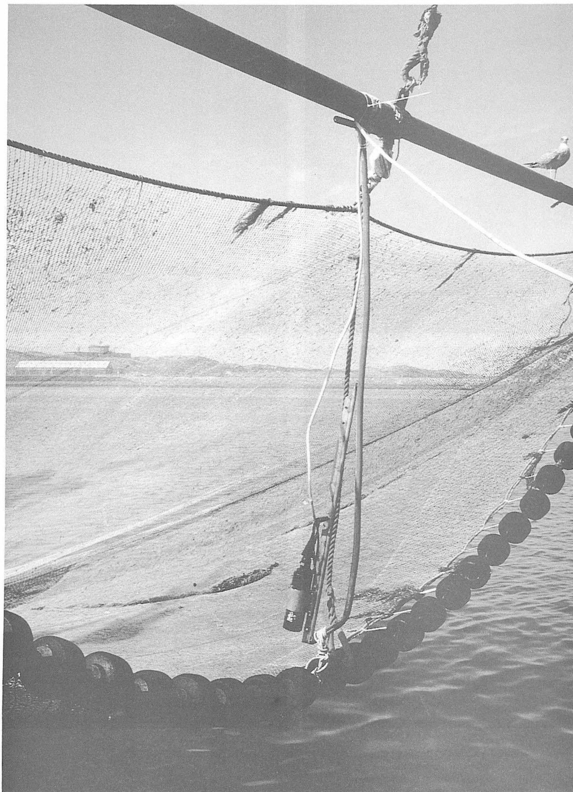
Fig. 8. Position of video-camera on mono-sled in the opening of 10 m shrimp trawl.
