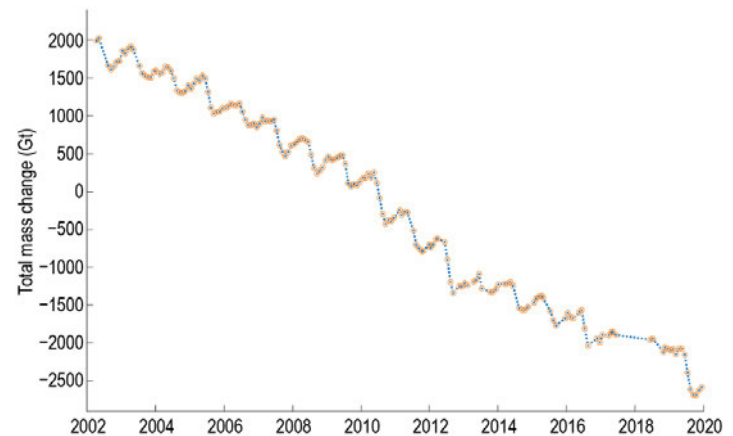
Fig. 5.15. Gravity-derived estimates (blue dots with yellow circles) of total mass change (Gt) of the GrIS between Apr 2002 and Dec 2019 determined from GRACE (2002–17) and GRACE-FO (2018–19) JPL RL06 Level 2 solutions (using techniques from Wahr et al. (1998); 2-std. dev. model fit uncertainties reported), with linear interpolation (blue dots). The following corrections have been applied: Geocenter (Technical Note 13); C20 and C30 (Technical Note 14); glacial isostatic adjustment (ICE-6G_D).
