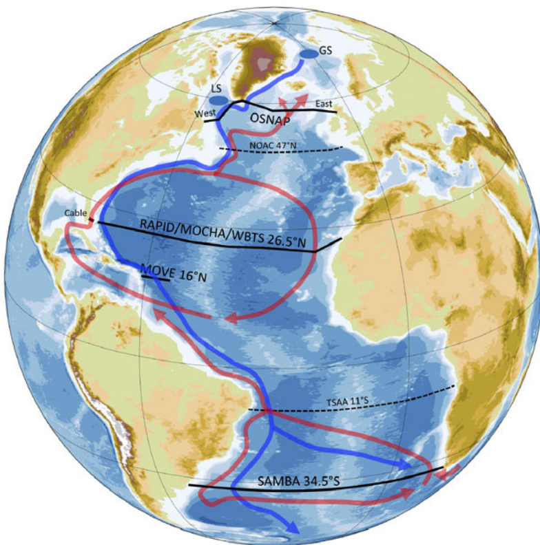
Fig. 3.20. AMOC continuous observing arrays producing transport estimates today (black lines) or expected to produce data soon (dashed lines). Arrows represent a simple schematic of the upper (red) and lower (blue) limbs of the overturning circulation. The conventional deep water formation regions in the Greenland (GS) and Labrador (LS) Seas are shown by blue-shaded circles.
